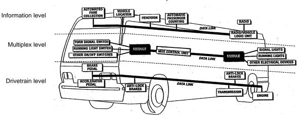
FIGURE 4 Data Communications Systems Levels
