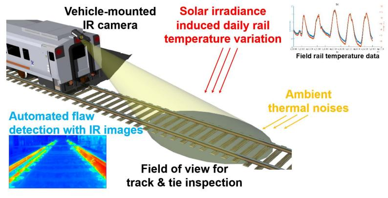
Figure 1- Concept of fully developed system for in-motion rail track and tie inspection
