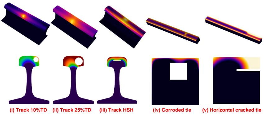
Figure 4. Full field and cross-sectional temperature distribution based on track and tie models
