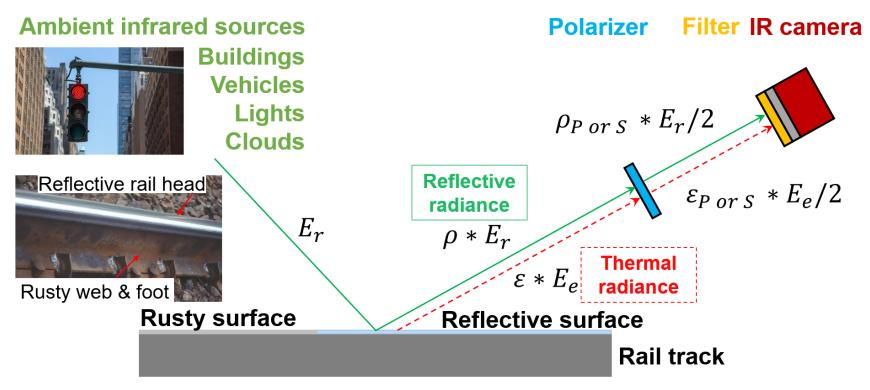
Figure 2 - Radiation energy detected by IR camera for rail track inspection
