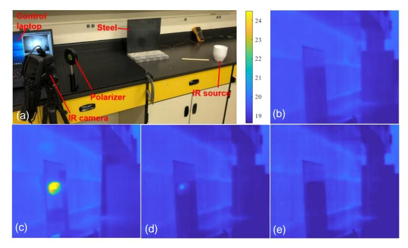
Figure 5. (a) Test setup for polarized IRT; temperature fields of steel plate (b) without IR source; (c) with IR source; (d) with IR source & polarizer; (e) with IR source & reflection compensation
